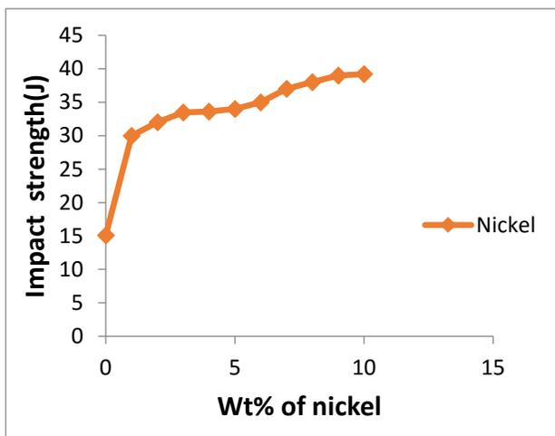
Figure 6. Effect of nickel content on the impact strength of Cu-10%Al alloy
