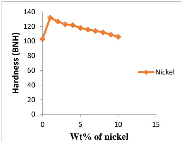
Figure 5. Effect of nickel content on the hardness of Cu-10%Al alloy
