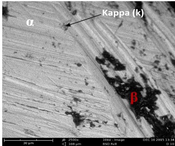
Figure 9: Plate 13: SEM micrograph of Cu-10%Al + 10%Ni
