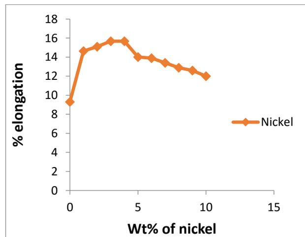
Figure. 4. Effect of nickel content on the % elongation of Cu-10%Al alloy
