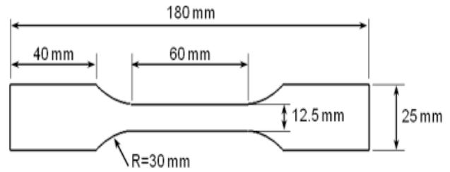
Figure 2: Tensile test specimens
