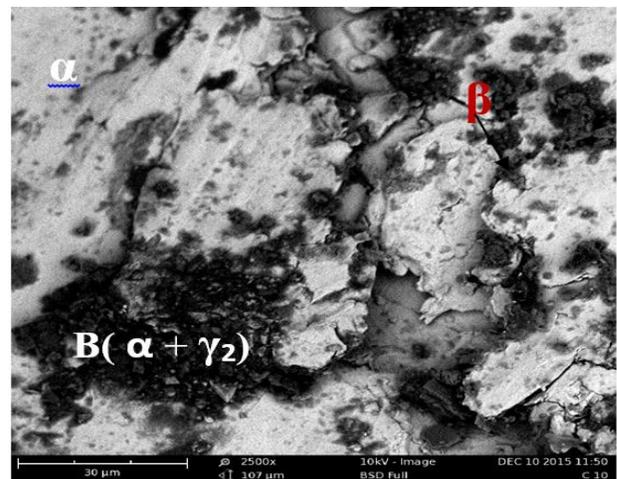
Figure 8: Plate 12: SEM micrograph of Cu-10%Al
