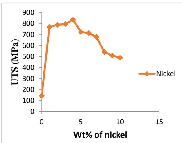
Figure. 3. Effect of nickel content on the UTS of Cu-10%Al alloy.
